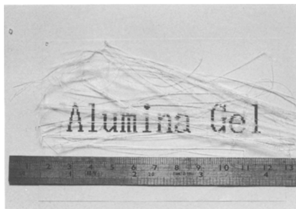
Figure 11 As-dried alumina fibre prepared by the aluminum nitrate system.
